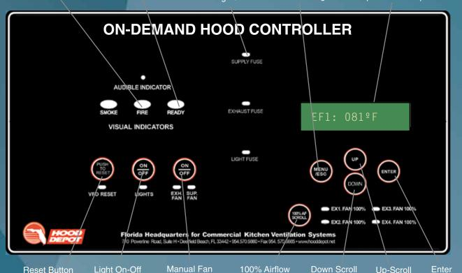
The controller varies the speed of the fans utilizing variable frequency drives that adjust speed from full speed down to a minimum speed (determined by menu setup). The system is capable of serving as an IMC 507.2.1.1 compliant auto start-up control to automatically start fans during cooking operations.
