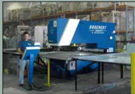
is a Boschert 1250, used to make an array of duplicate parts to exact tolerances of our CNC KAD software, interfaced with our engineering department software, which draws from our Reddit 3D modeling program.
